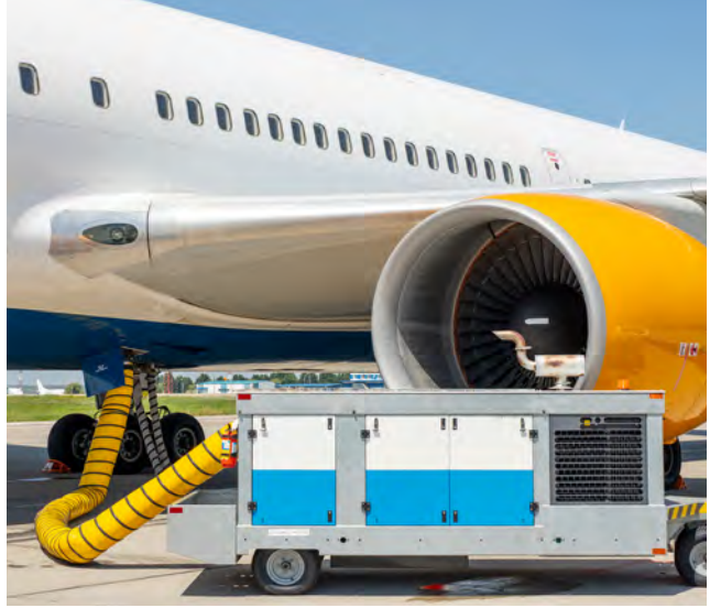
Görsel 3.5: Air Condition Unit (ACU)
