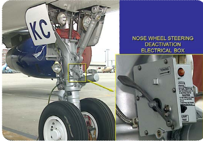
Görsel 3.6: Nose wheel steering deactivation electrical box
