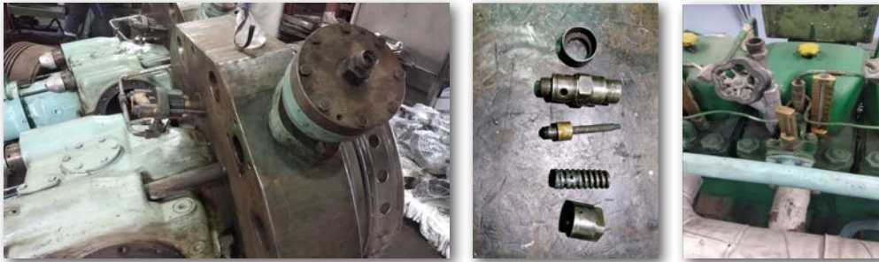
Görsel 3.11: Starting valf, rilif (safety) valf ve termometre
